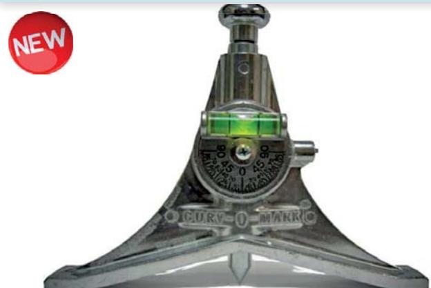
The central engraver is used for tubes starting from diameter of cm. 2.5 and over. In the engraver there is an adjustable stop rod and a protractor with bubble. After having extracted it to the stop point and after having leveled the engraver, release the rod by pressing the locking spring. The pressure exerted on the rod will strongly hit the tube marking the center. **Packing:** 1 pz.
