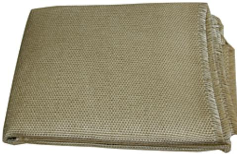
Heat-resistant fiberglass blanket, medium-wide weave, 2mm thick, weight 1155g / m<sup>2</sup>. Sand color. Serving temperature 450 ° C, limit 600 ° C.
